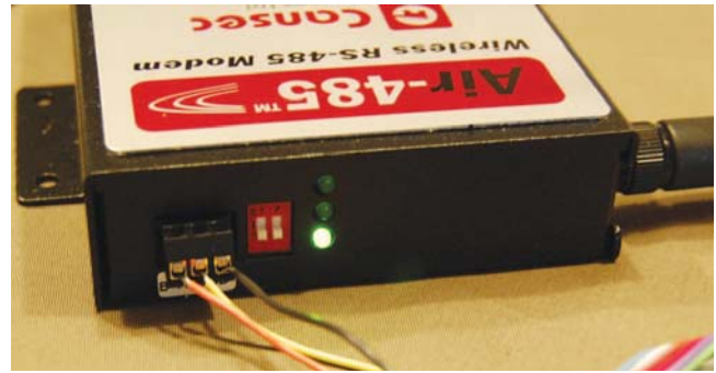
19. The other end has a signal strength meter and RS-485 connection.
