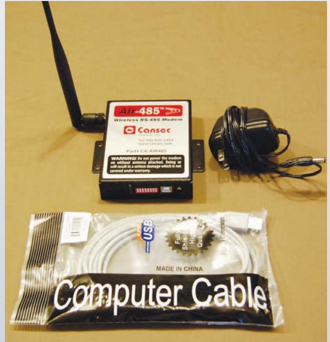
17. Here is the Air-485® wireless modem with a range of up to 6 miles.
