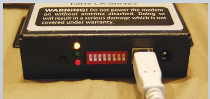
18. One end has the USB connection and indicator lights.
