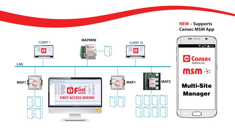
Cansec's First Access® software provides a powerful yet easy to use platform to manage the whole family of MAP access control panels. It is available in two versions: The free Express version for basic access control functions and Advanced for more complex applications. Both support up to 1,024 readers and 100,000 cards. NEW - First Access Advanced software now support the Cansec MSM app which allows you to control and manage your system from anywhere.
